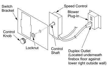
Figure 26 - Attaching Speed Control to Firebox
